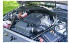
It's powered by a longitudinallymounted 2.0L turbocharged fourcylinder gasoline engine, paired up
